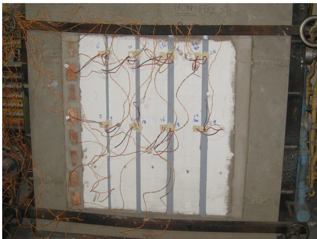
The unexposed face of the wall construction after 60 minutes of testing
