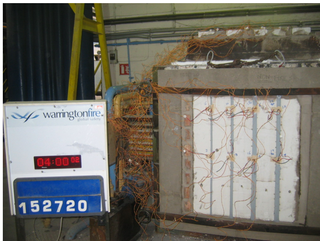
The unexposed face of the wall construction after 240 minutes of testing
