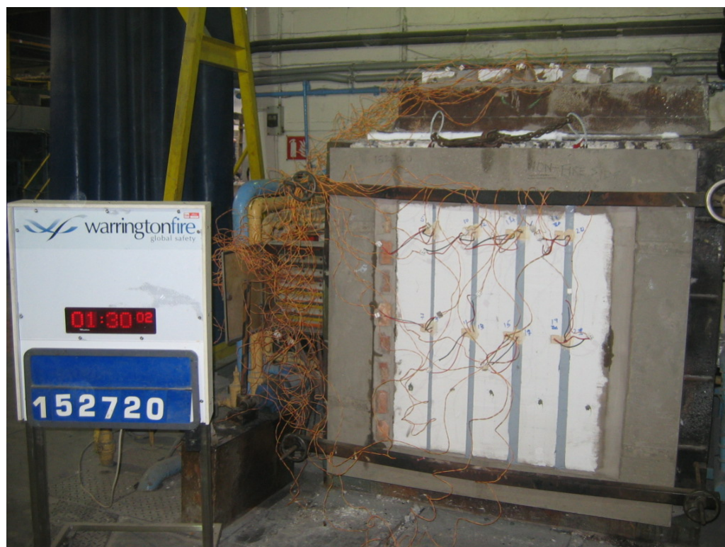
The unexposed face of the wall construction after 90 minutes of testing
