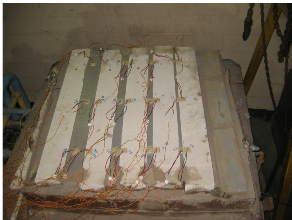
The unexposed face of the floor construction after 90 minutes of testing
