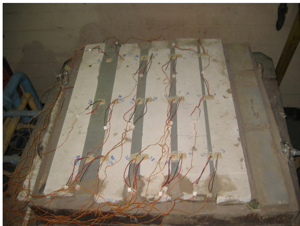
The unexposed face of the floor construction after 240 minutes of testing
