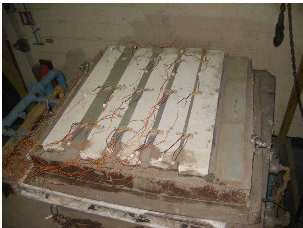
The unexposed face of the floor construction after 120 minutes of testing
